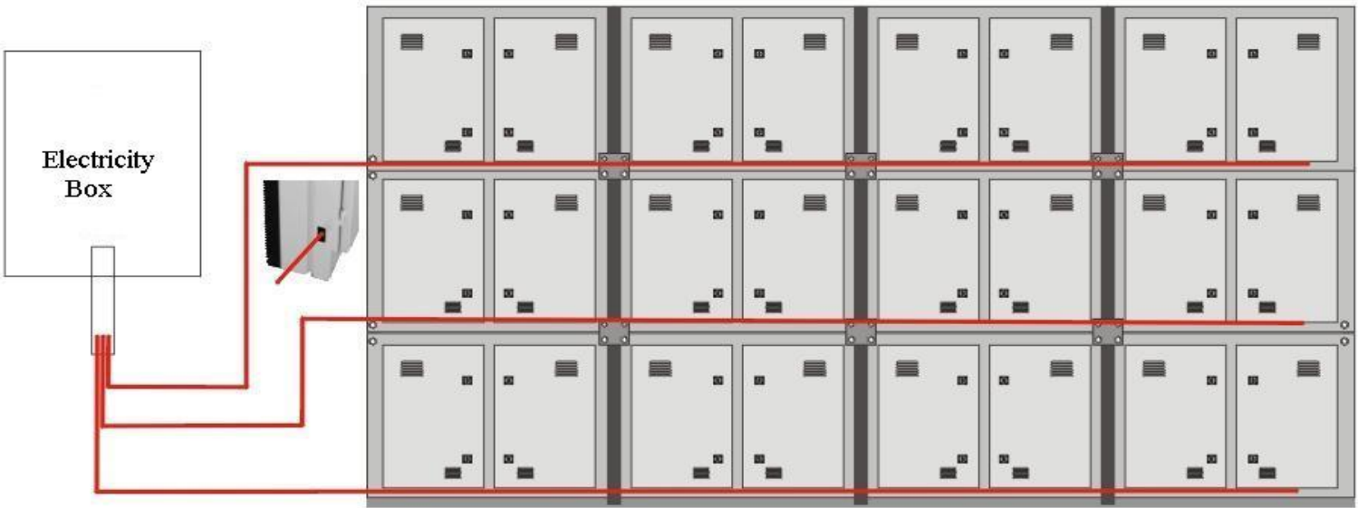
Power Line Connection Diagram between up and down cabinets
