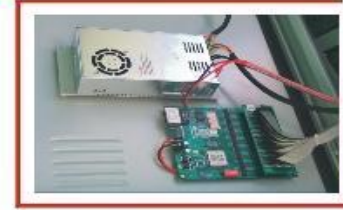
Power supply from AC to DC current
